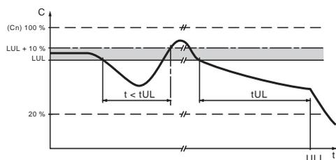
Motor underload detection (ULL)
