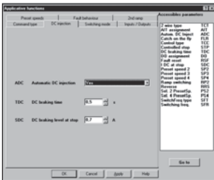
Adjustment of the "d.c. injection" function using the PowerSuite software workshop for PC
