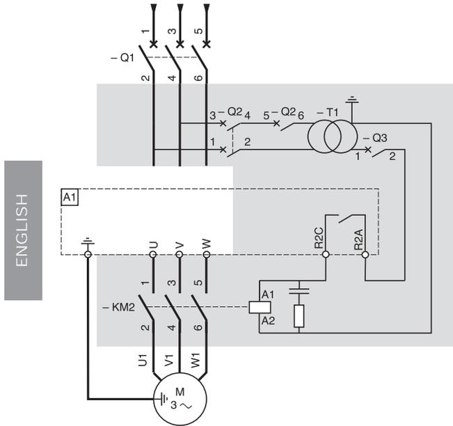
Use the "downstream contactor control" function with relay R2, or logic output LO ( $\sim$ 24V) switching the coil using an I/O extension card. Consult the programming manual.
