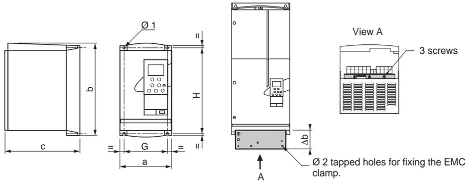
The EMC mounting plate is supplied with clamps for ATV38HU18N4 to D79N4(X) drives. Fix the EMC equipotentiality mounting plate to the holes in the ATV38 heatsink using the screws supplied, as shown in the drawings above.
